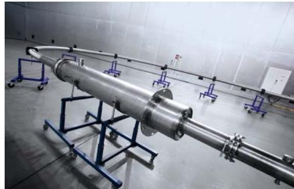
This prototype of a superconductive cable system for Essen city centre was put through its paces in the high-voltage laboratory in Nexans' Hanover plant.
